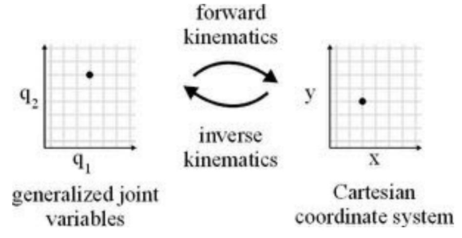
Forward kinematics: based on joint angles, calculate endeffector position
