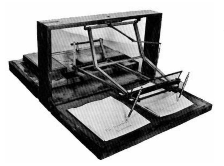
A Polygraph is a device that produces a copy of a piece of writing simultaneously with the creation of the original, using pens and ink.
